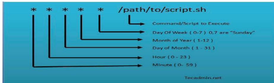
Figure 3 Crontab structure.(command to be executed)
