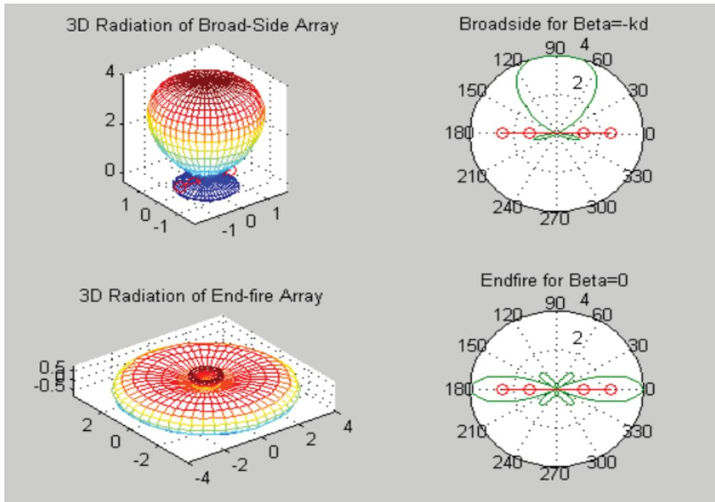
Figure 3: Simulation of 3D& 2D Radiation pattern of Broadside and End fire array
