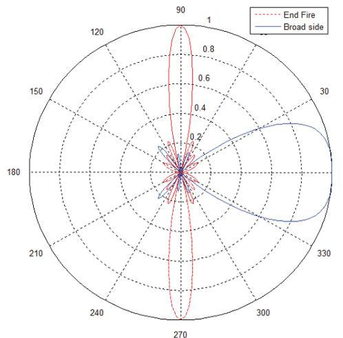
Figure:4 Radiation pattern in polar co ordinate
