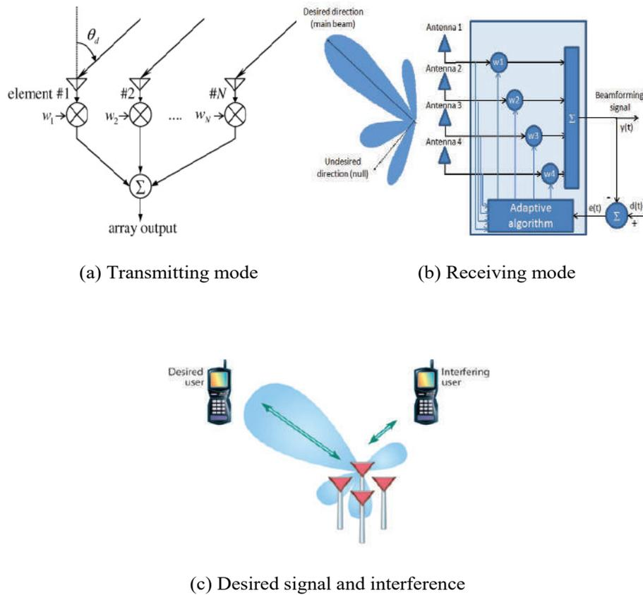
Figure 2. Array antenna beam former including desired signal and interference
