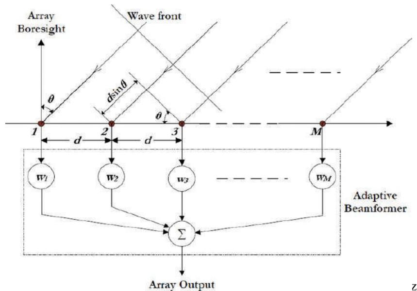
Figure :1 Linear array antenna with adaptive filter
