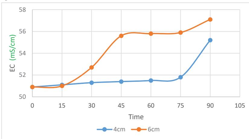
Figure 10: Effect of operating time and electrode spacing on Electric Conductivity.
