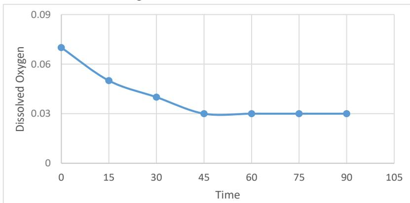
Figure 8: Effect of operating time on DO (4 cm electrode spacing).
