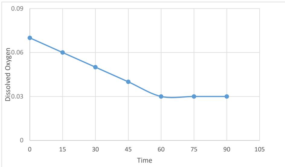
Figure 9: Effect of operating time on DO (6 cm electrode spacing).
