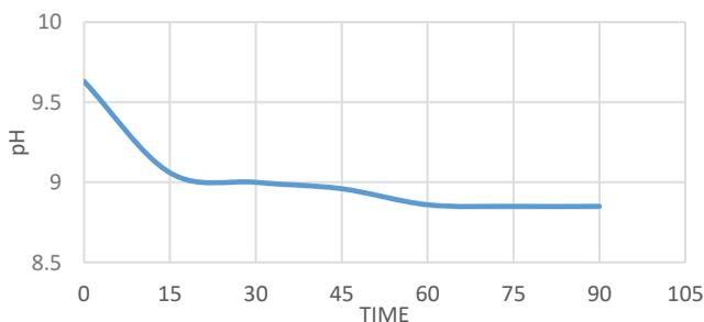
Figure 5: Effect of operating time on pH (6 cm electrode spacing).
