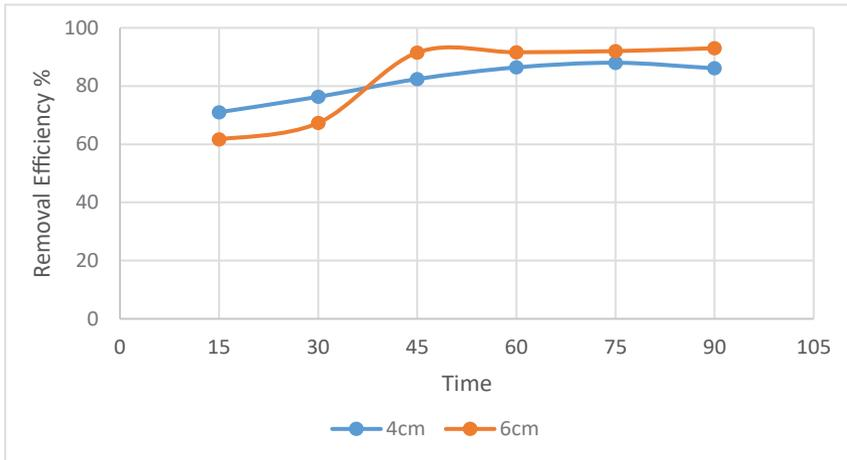
Figure 6: Effect of operating time and electrode spacing on removal efficiency of color.
