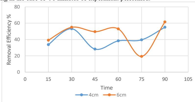
Figure 7: Effect of operating time and electrode spacing on removal efficiency of COD.
