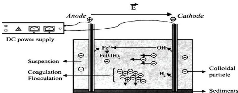
Figure 1: Principle of electro coagulation process.
