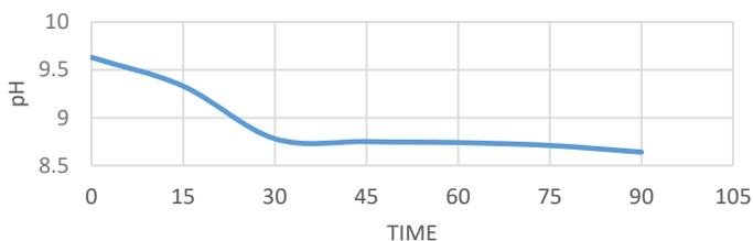
Figure 4: Effect of operating time on pH (4 cm electrode spacing).
