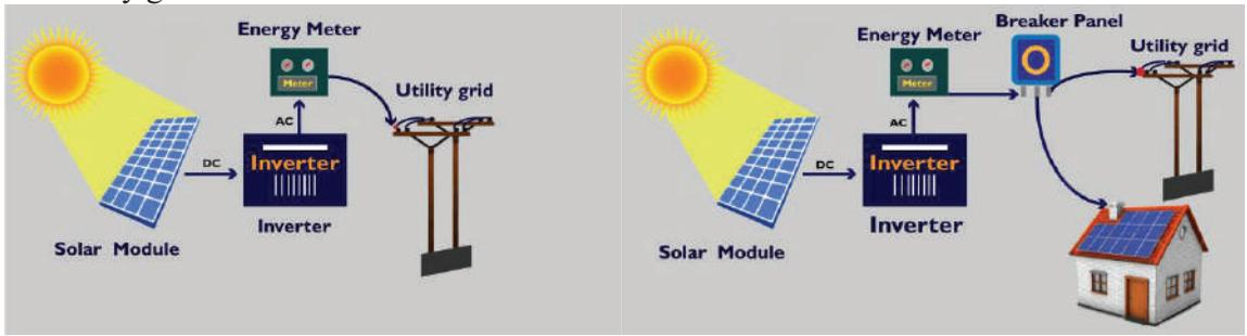
Figure 2. (a). Battery less PV Grid-Tie System Solely Connected to Utility Grid (b). Battery less PV Grid-Tie System Connected to Utility Grid and Home Appliances
