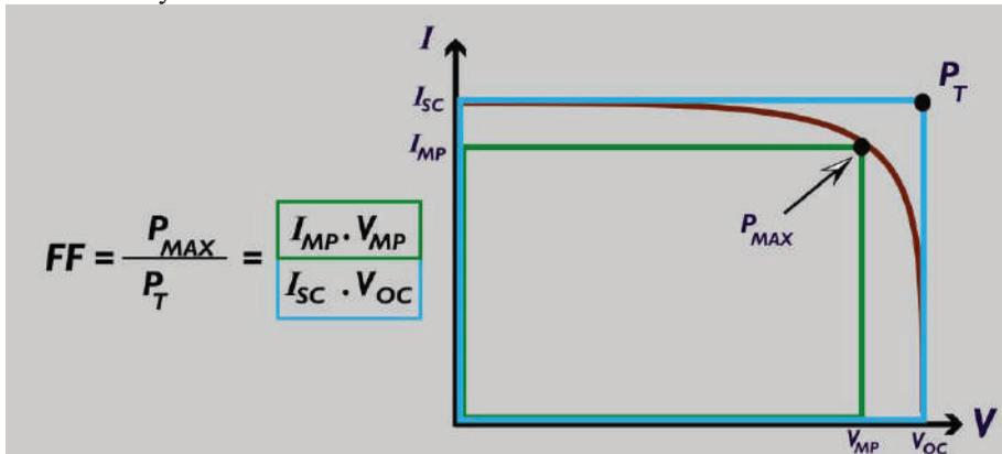
Figure 1. Fill factor and Efficiency
