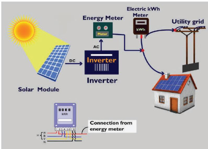
Figure 3. Implemented Grid-Tie System.
