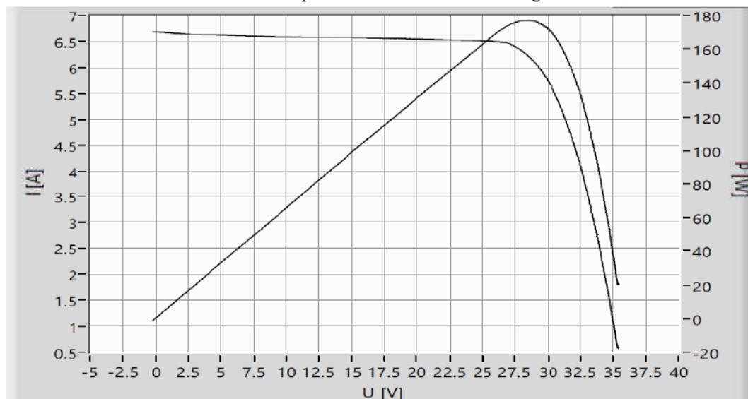
Figure 4. I-V and P-V curves of 260 W polycrystalline solar panel
